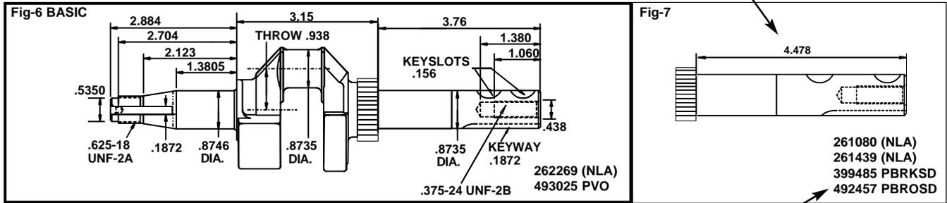
To order the crankshaft, the service number is located in the lower right hand corner of each box. If there is more than one service number listed, the part has been superseded. Review the other part number(s) listed. Check the abbreviations behind the number to determine the correct crankshaft.
