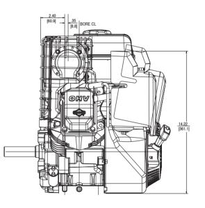
To make the center line of crankshaft the same as 190000 and 250000 Model Series, order 695154 spacer kit.
