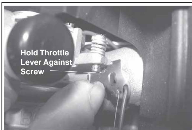
Figure 21. Holding Throttle Lever Against Idle Stop Screw.
