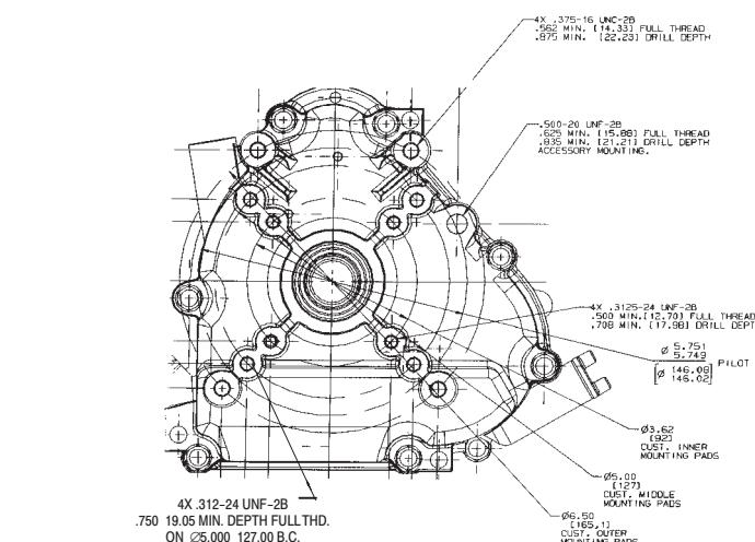
To make the center line of crankshaft the same as 190000 Model Series, order 695154 spacer kit.
