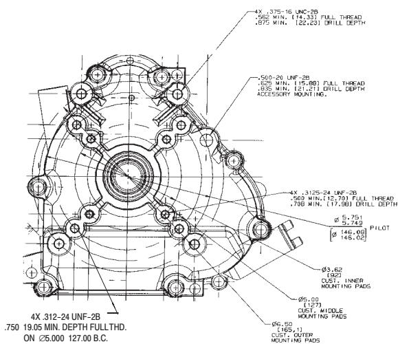
To make the center line of crankshaft the same as 190000 Model Series, order 695154 spacer kit.
