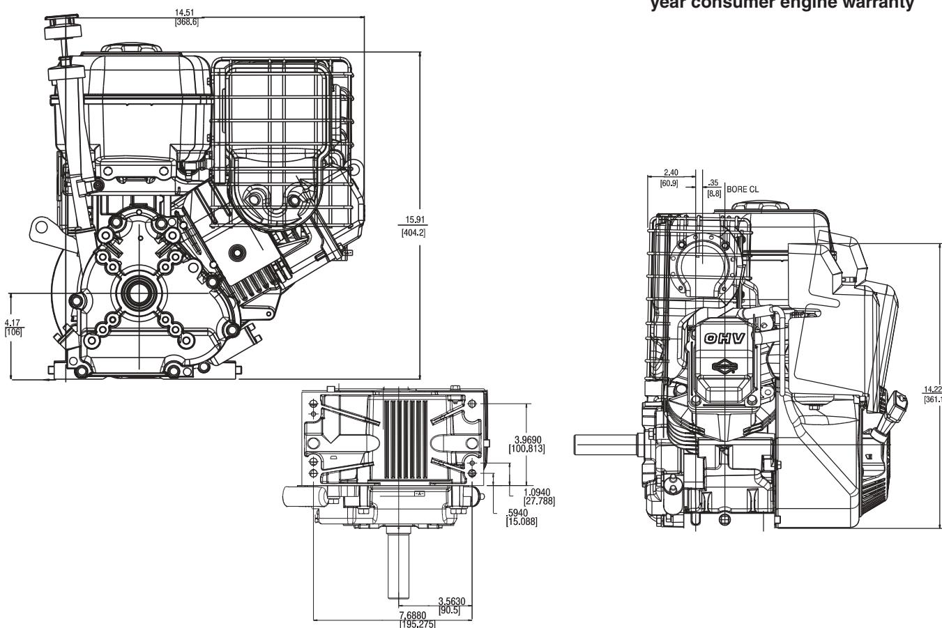
To make the center line of crankshaft the same as 190000 and 250000 Model Series, order 695154 spacer kit.
