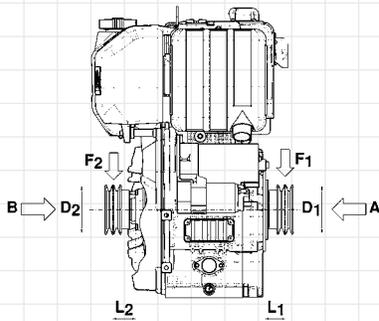
$$D_1 \text{ (mm)} \geq 620 [66 + L_2 \text{ (mm)}] \frac{N \text{ (kW)}}{n \text{ (RPM)}}$$
