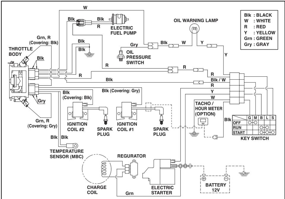
Optional hardware shown by dotted lines. Select wires of proper gauge and connect battery as shown by the dotted line in the wiring diagram.
