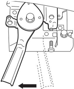
Gradually move the speed control lever toward the high speed position and set it at the required engine speed.
