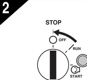
Turn the key switch to the "STOP" position.
