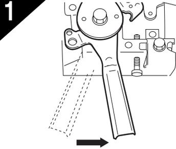
Set the speed control lever at the low speed position and allow the engine to run at low speed for 2 or 3 minutes before stopping.
