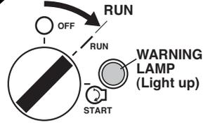
If there is a control box mounted, turn the key switch and set it to the "RUN" position. Check to make sure that the warning and other lights illuminate (red).
