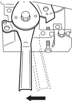
Set the speed control lever 1/3 of the way towards the high speed position.
