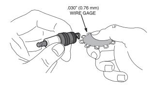
Note: In some areas, local law requires using resistor spark plug to suppress ignition signals. If this engine was originally equipped with resistor spark plug, use same type for replacement.
