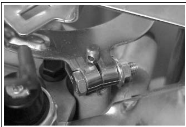
Figure 5B-38. Checking "Split" of Clamp.
