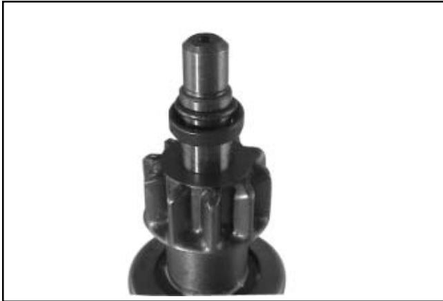
Figure 8-49. Retaining Ring Detail.
