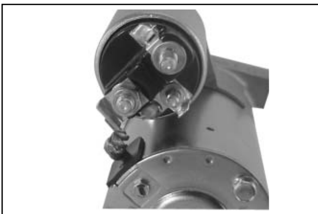
Figure 8-69. Positive (+) Brush Lead Connection.
