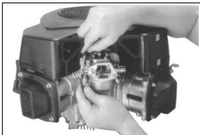
Figure 11-69. Installing External Governor Controls.
