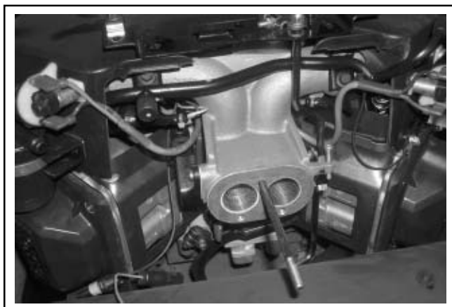
Figure 5B-32. Upper Throttle Body/Intake Manifold Details.
