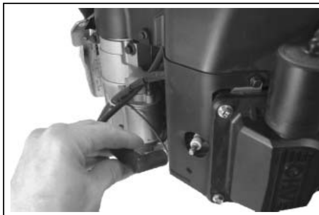
Figure 9-1. Disconnect Spark Plug Leads.
