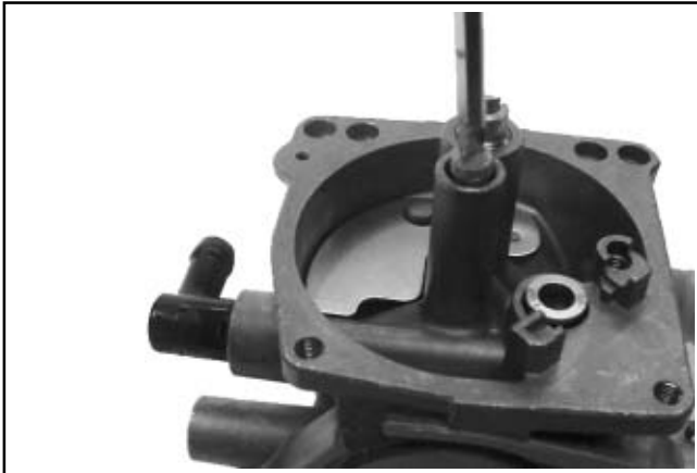
Figure 5-18. Installing Slow Jet.
