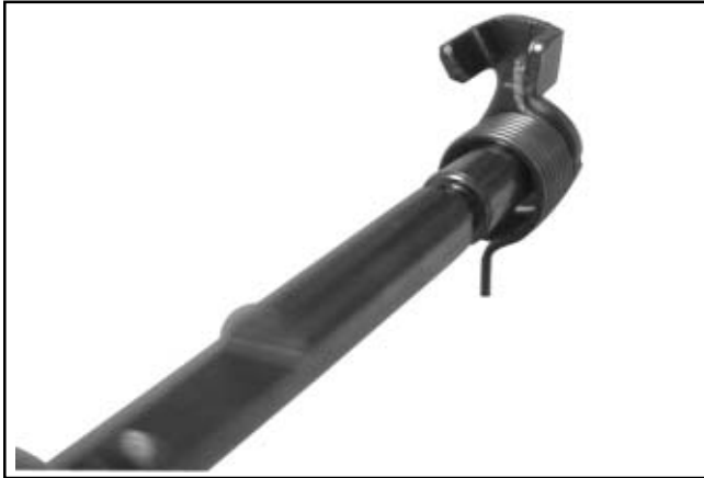
Figure 5-35. Choke Shaft and Spring Details.
