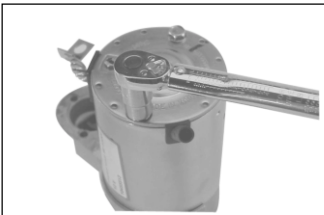
Figure 8-67. Torquing Thru Bolts.
