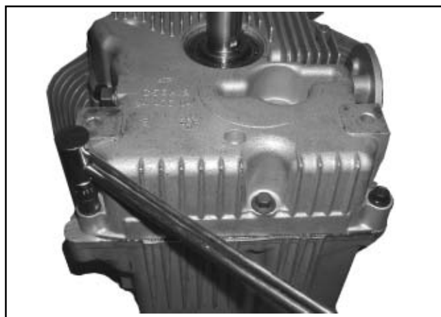
Figure 11-19. Torquing Oil Pan Fasteners.
