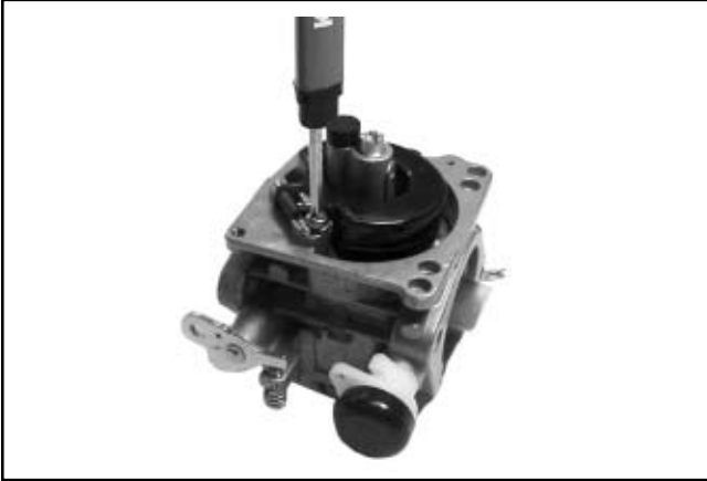
Figure 5-11. Installing Float Assembly.
