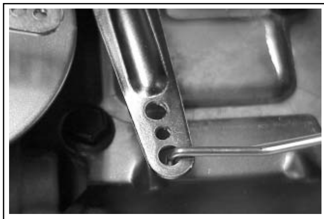
Figure 5B-37. Throttle Link in Center of Hole.
