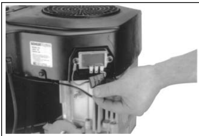
Figure 11-65. Attaching Connector Plug.
