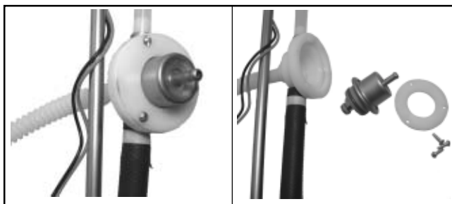
Figure 5B-28. Internal (In-Tank) Regulator and Base/Holder.
