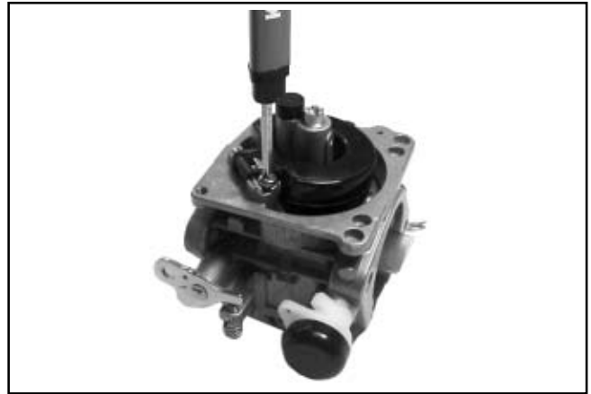
Figure 5-21. Installing Float Assembly.
