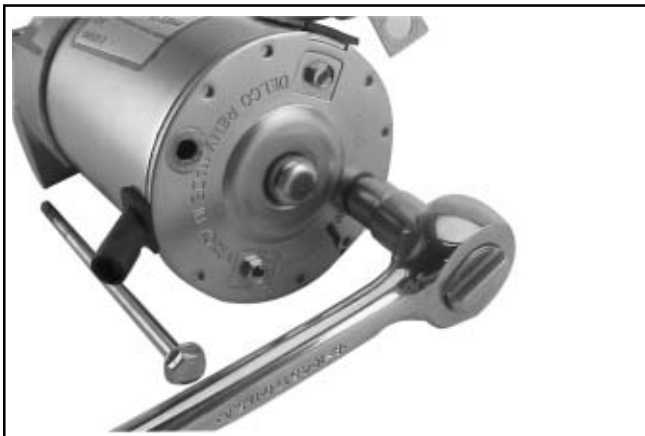
Figure 8-44. Removing Thru Bolts.
