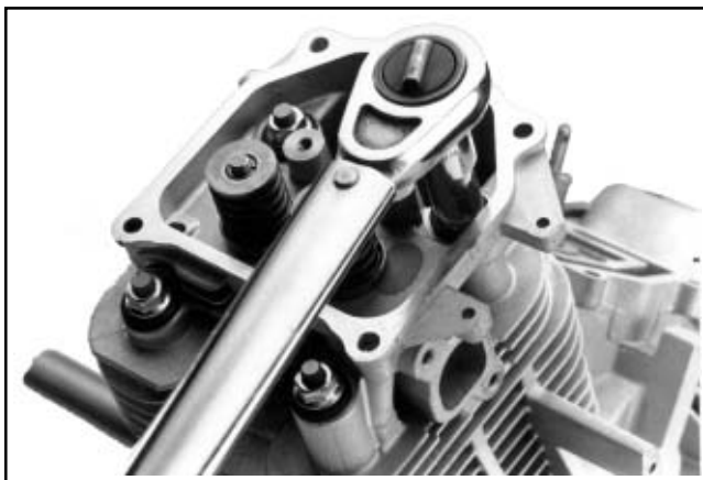
Figure 11-40. Torquing the Cylinder Head Mounting Nuts (Stud Design).
