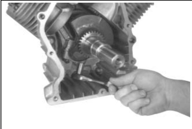
Figure 9-54. Removing Connecting Rod End Cap.
