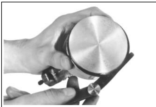
Figure 10-10. Measuring Piston Ring Side Clearance.
