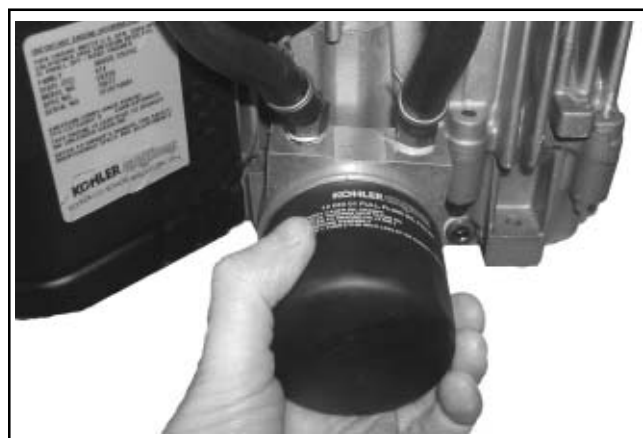
Figure 11-83. Installing and Tightening Oil Filter.
