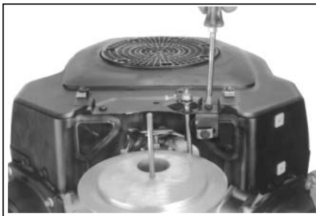
Figure 11-71. Installing Control Panel.
