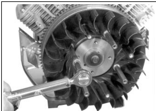
Figure 11-29. Torquing Supports for Metal Screen (Some Models).
