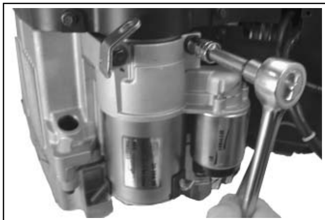
Figure 9-19. Removing Electric Starter Motor.
