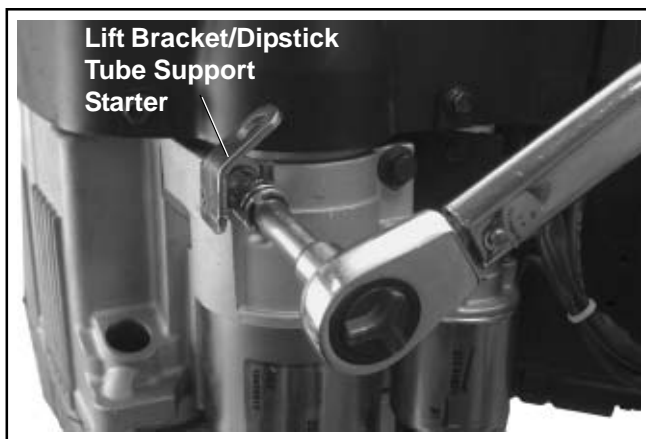
Figure 11-75. Installing Starter and Lift Bracket.
