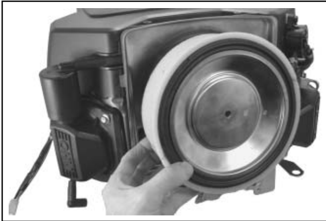
Figure 9-6. Removing Standard Element and Precleaner.
