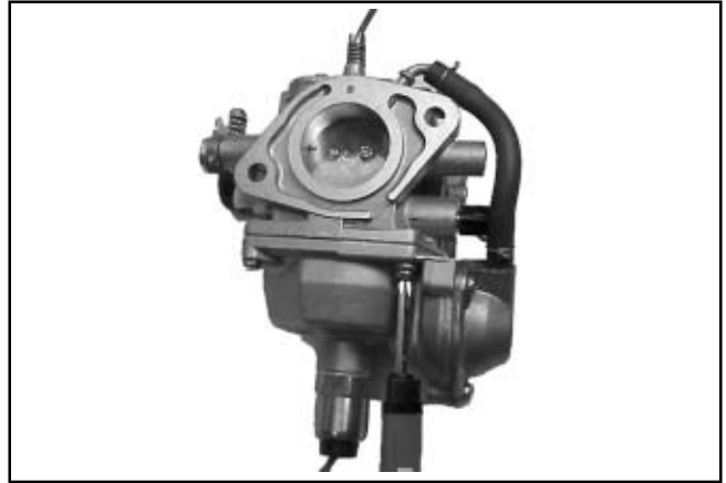
Figure 5-13. Installing Fuel Bowl.
