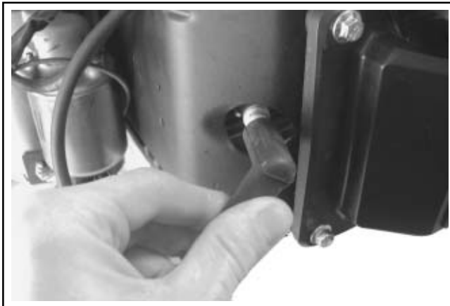
Figure 11-85. Connect Spark Plug Leads.
