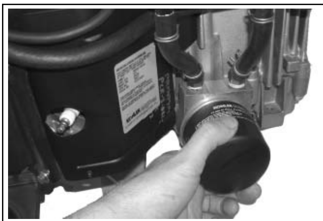
Figure 9-4. Removing Oil Filter.
