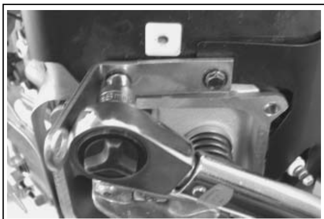
Figure 11-60. Tightening Outer Baffle Front Screws.
