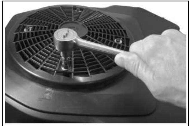
Figure 9-24. Removing Flywheel Screen.
