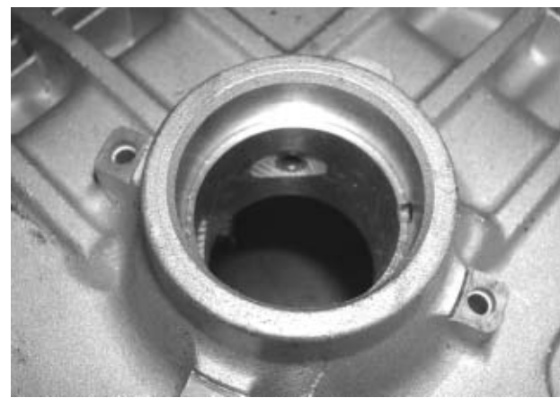
Figure 11-1. Seal Bore of Crankcase.
