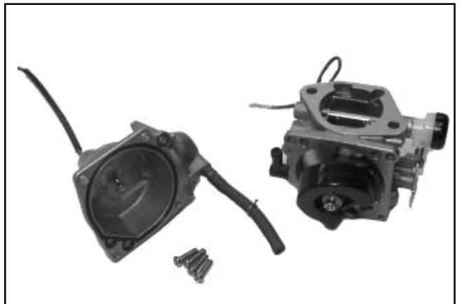
Figure 5-14. Fuel Bowl Removed from Carburetor.
