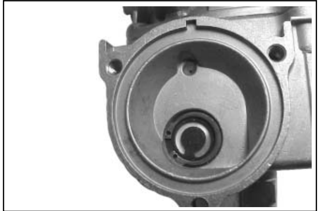
Figure 5-29. Check Valve and Retaining Ring Installed.
