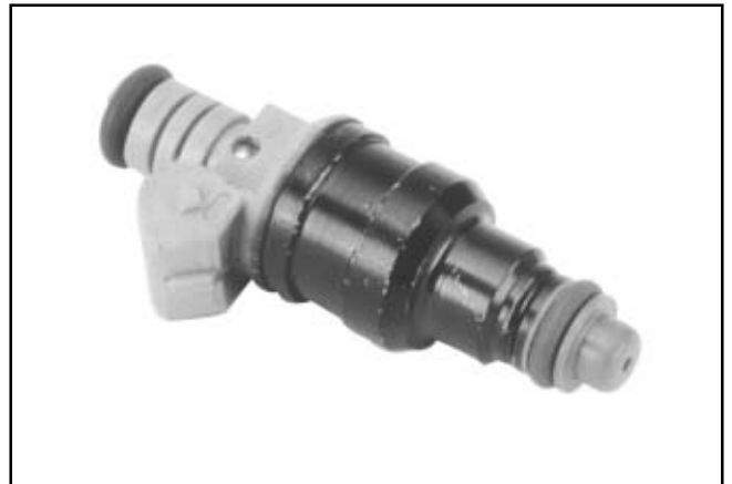
Figure 5B-14. Style 1 Fuel Injector.
