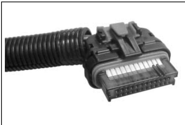
Figure 5B-21. “24 Pin” (MSE 1.0) Plastic-Cased ECU Connector.
