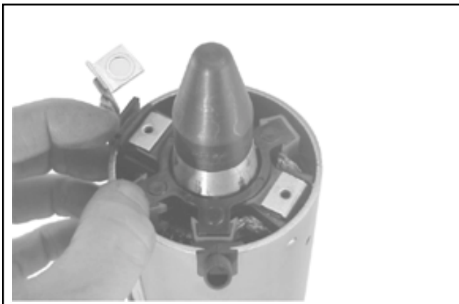
Figure 8-66. Installing Brush Holder Assembly using Tool with Extension.
