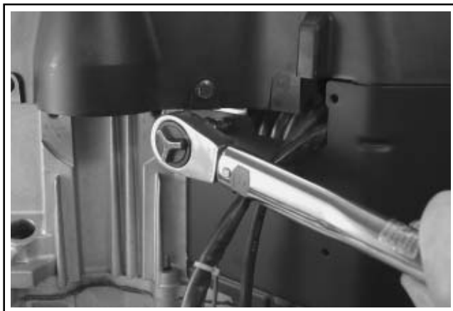
Figure 11-61. Tightening Short Screws for Outer Baffles.
