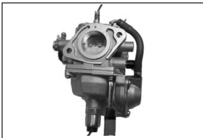
Figure 5-24. Installing Fuel Bowl.
