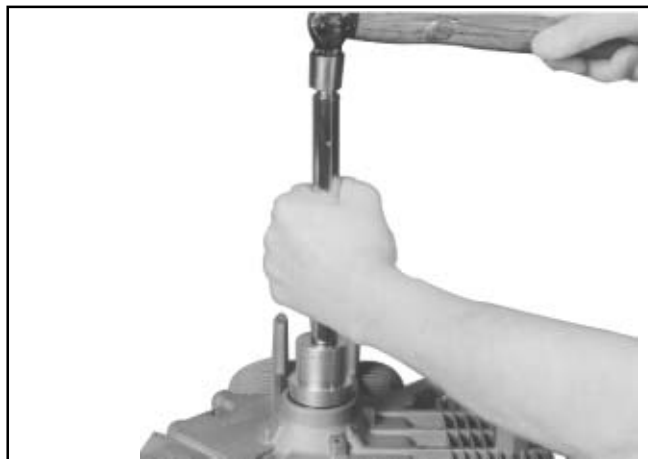
Figure 11-2. Installing Oil Seal in Crankcase.
