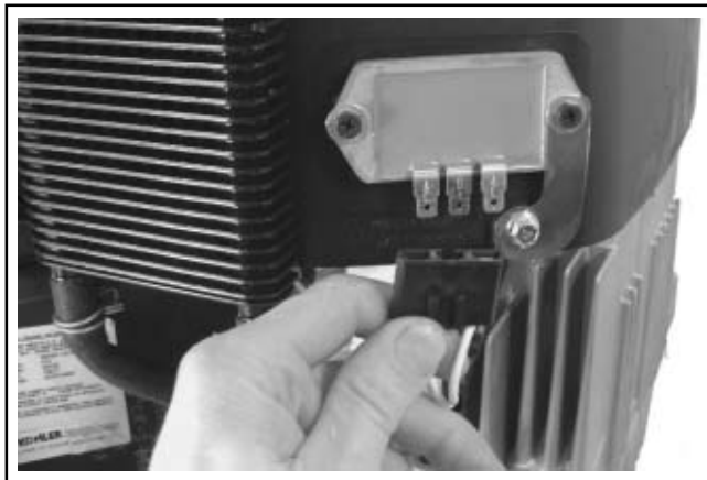
Figure 9-20. Disconnecting Plug from Rectifier-Regulator.
