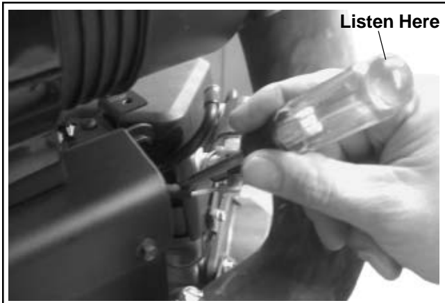
Figure 5B-17. Checking Injectors.
