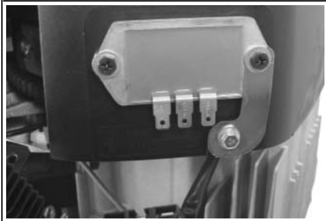
Figure 11-64. Rectifier-Regulator Ground Details.
