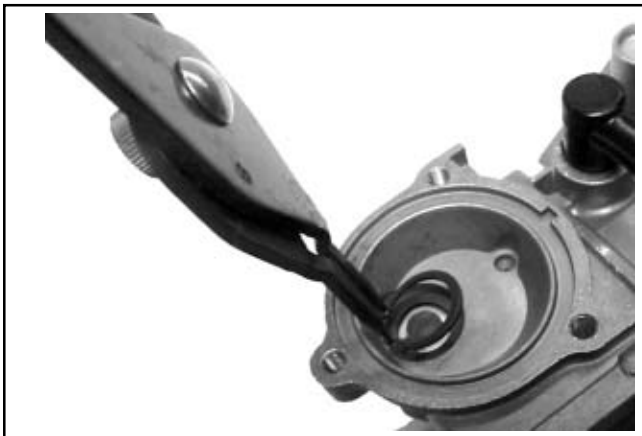
Figure 5-28. Removing Retaining Ring.
