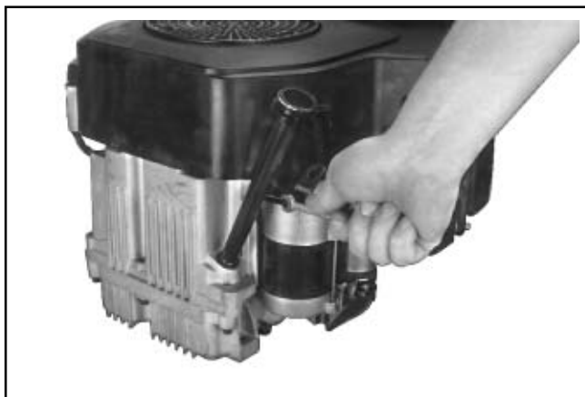
Figure 9-3. Removing Oil Fill Tube Bracket.
