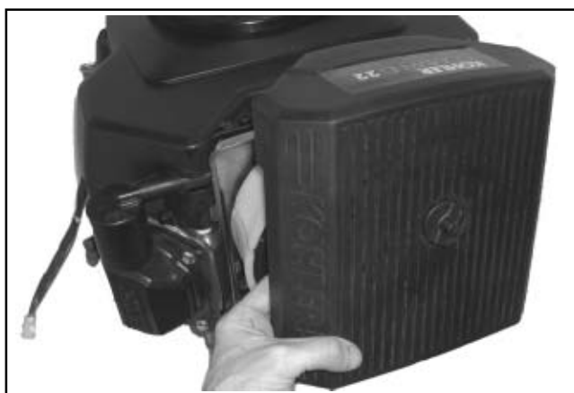
Figure 9-5. Removing Standard Air Cleaner Cover.
