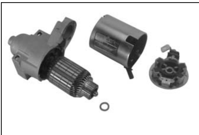
Figure 8-46. Starter Frame Removed.
