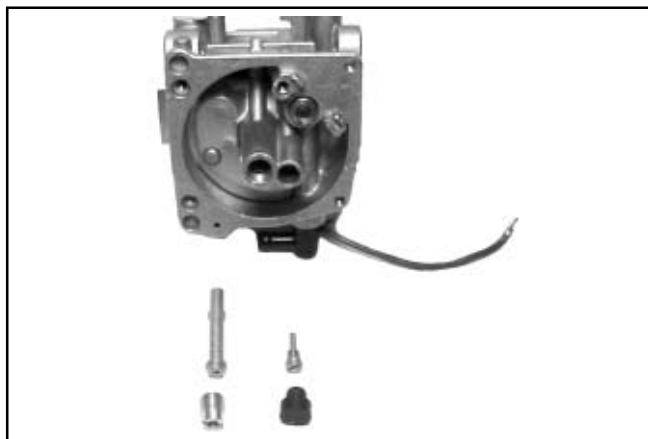
Figure 5-16. Main Jet and Slow Jet Removed.
