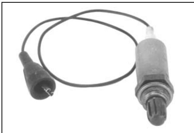
Figure 5B-9. Oxygen Sensor.
