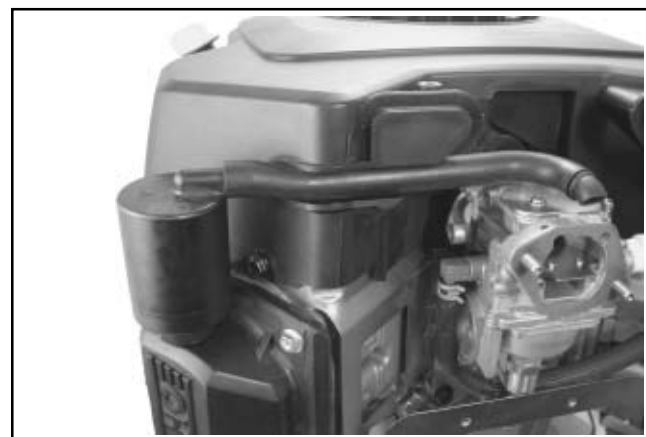
Figure 11-80. Breather Hose and Separator Details.
