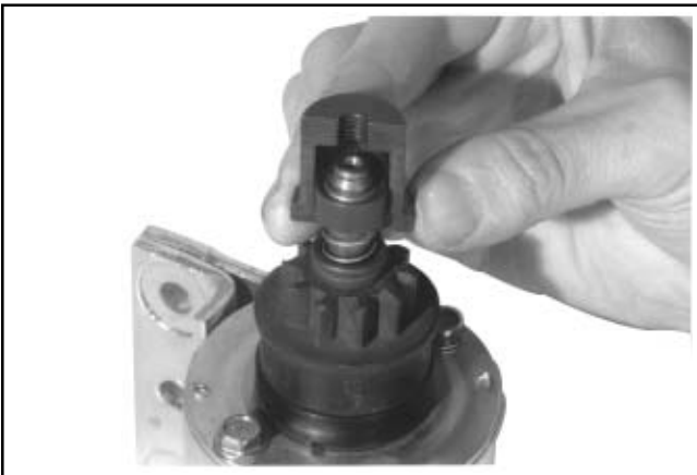
Figure 8-34. Assembling Larger Inner Half Around Spring Retainer.
