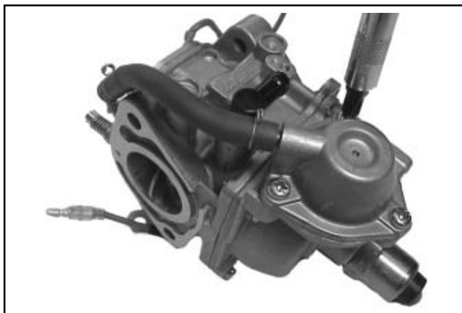
Figure 5-31. Installing Accelerator Pump Housing Screws and Hose.
