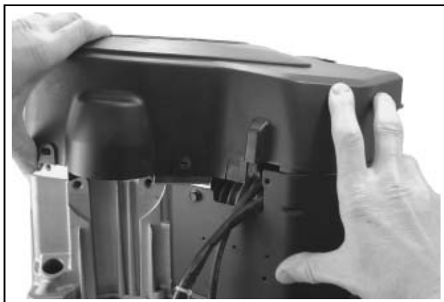
Figure 11-59. Installing Blower Housing.
