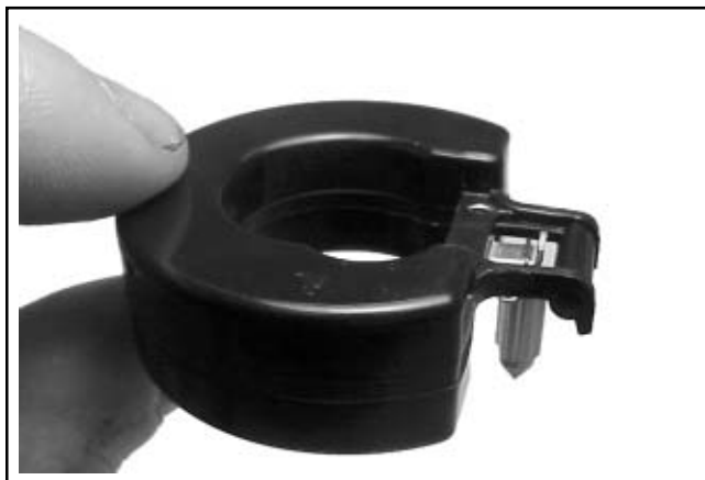
Figure 5-20. Float and Inlet Needle.
