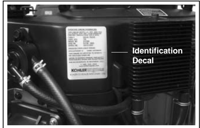
Figure 1-1. Engine Identification Decal Location.
