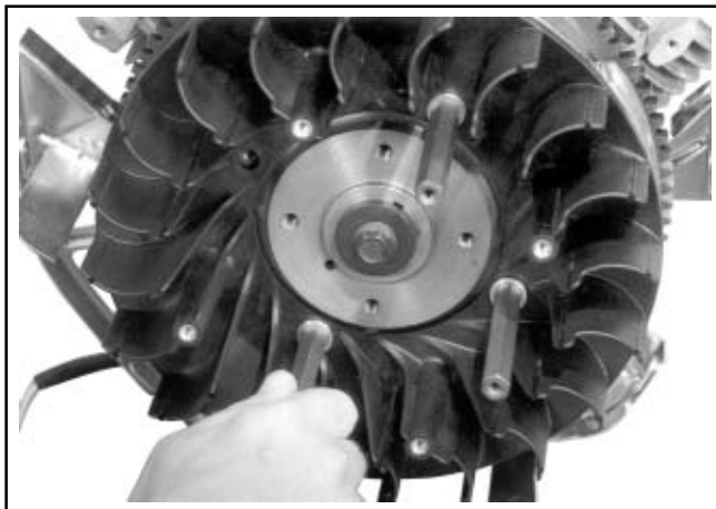
Figure 11-28. Installing Supports for Metal Grass Screen.
