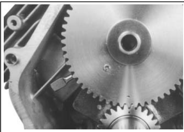
Figure 11-13. Aligning Crankshaft and Camshaft Timing Marks.
