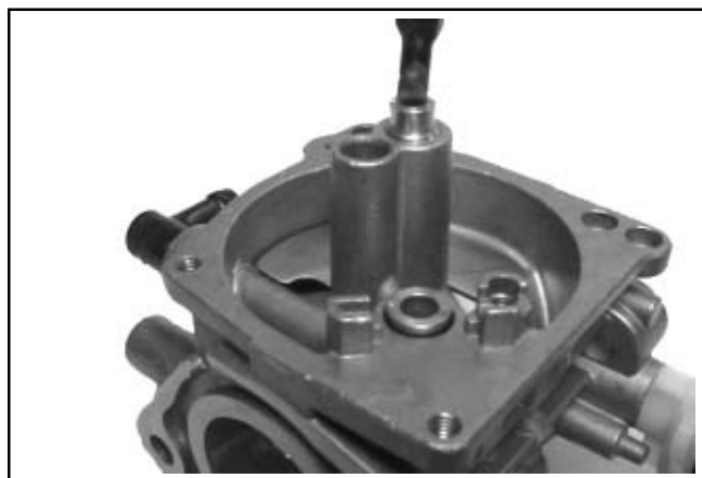
Figure 5-17. Installing Main Nozzle and Main Jet.
