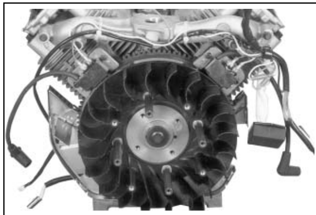
Figure 8-6. Capacitive Discharge Ignition System with Spark Advance.
