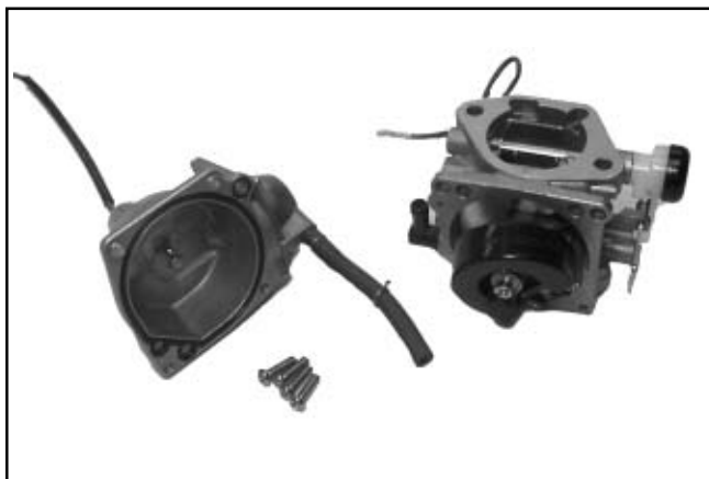
Figure 5-8. Fuel Bowl Removed from Carburetor.
