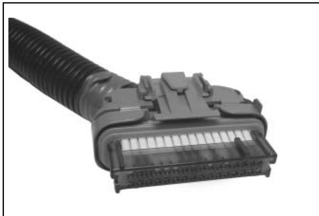
Figure 5B-22. “32 Pin” (MSE 1.1) Plastic-Cased ECU Connector.
