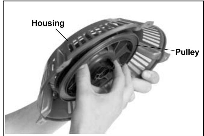
Figure 7-6. Removing Pulley from Housing.
