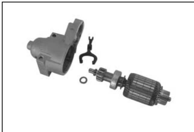
Figure 8-48. Armature and Lever Removed.
