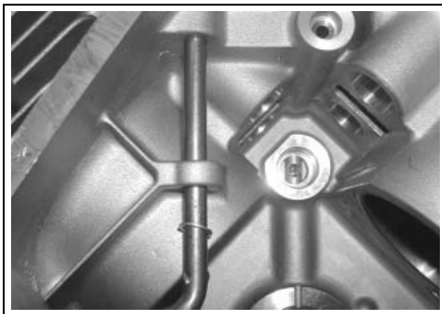
Figure 11-5. Installing 8 mm Governor Cross Shaft.
